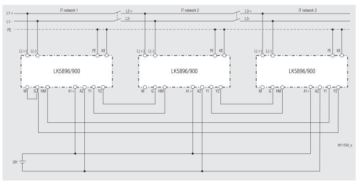
Monitoring of 3 separate DC voltage systems, that can be coupled by coupling switches. By sequential triggering of the insulation monitors it is made sure that only one of the insulation monitor is active at the same time. the first insulation monitor in IT network 1 is configured as master and starts the measuring cycle after power up. To provide synchronous starting of all insulation monitors in a system we recommend to use the same same source for the power supply UH.
