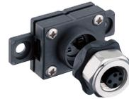
AS-Interface cable connector, used for distribution of connections or as connector: reusable access technology to IEC 68 and DIN 41611, hexagon screw in stainless steel, 4 poles. AS-Interface connector 0911 ANC 415 is included with the delivered product.
