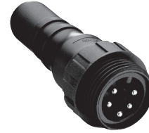
DeviceNet terminating resistor, 7/8" male connector, 5 poles.
